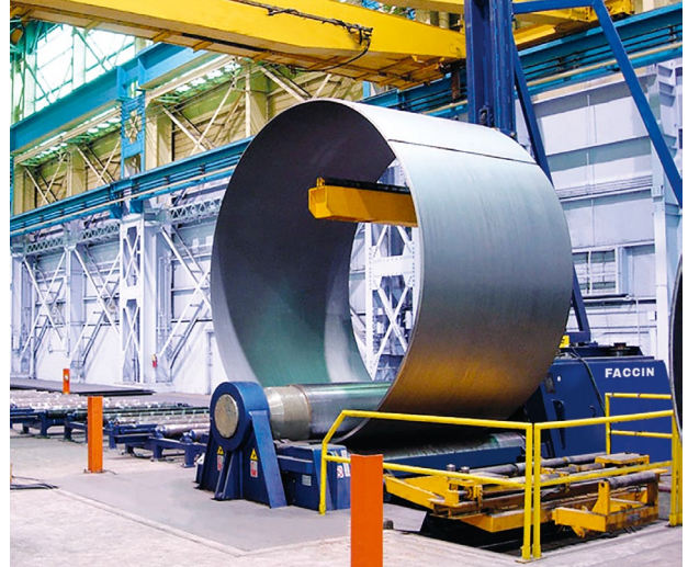
Faccin machines have a floor-to-floor production time of 20 minutes for each tube.
