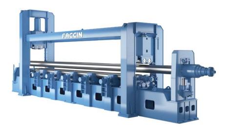
Faccin has many years of experience in the design and manufacturing of special machines for the production of pipes. To meet specific production requirements in the industry, the company offers HAV-2P, a series of high-performance pipe mill bending rolls able to support the production of pipes delivering productivity, repeatability and automation of the entire process.
