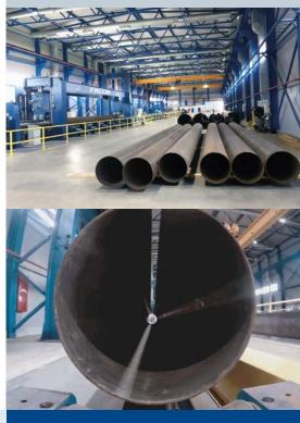
HAV-2P bending rolls are designed for rolling plates up to 45 mm thick, ideal for producing pipes up to over 18 m long, complying with certain technical specifications and roundness tolerances and offering a high-quality finished product complying with API standards.
