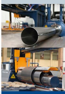
The standard HCU machine can guarantee output levels of 180-200 pieces/hour while the special version HCU/S reaches output levels beyond 300 pieces/hour.
