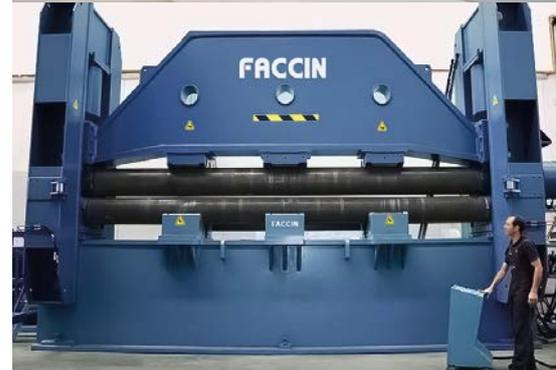
Faccin has designed a range of solutions able to meet the production requirements of the shipbuilding and aerospace industries. RP 3-Roll bending roll is a line of over-dimensioned bending rolls with force up to 3000 metric tonnes designed to bend plates wider than 20 meters. The special machines are able to effectively combine the production speed of a bending roll with the versatility of a press brake.
