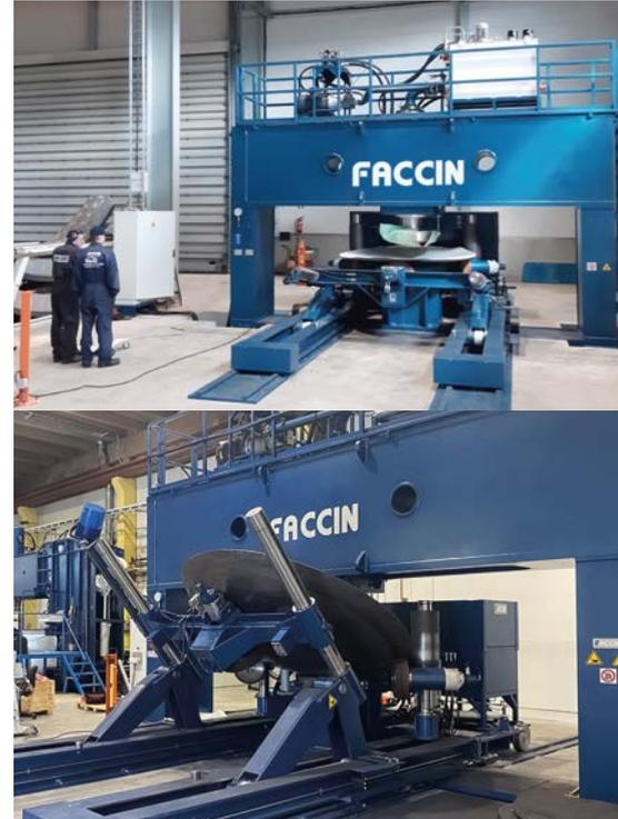
PPM is the series of sturdy, reliable and efficient Faccin hydraulic presses. Those designed and built by Faccin are presses suited to dished head crowning, featuring an exclusive design with rods and available in various sizes. To choose the exact size it is necessary to calculate the development of the largest dished end to be produced that indicates the distance between the uprights. The maximum thickness will guide the choice of the machine force.
