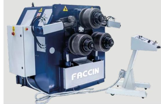
The RCMI series "double pinch" angle rolls are expressly designed for rolling profiles with high resistance to the process.
