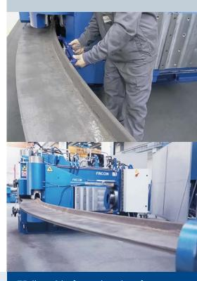
FB line ship frame benders feature full automation of the complete process thanks to the optional numerical control units (CNC). The CNC is automatically handling the feeding of the profile and the movements of the bending arms for the complete automatic and operator-free process.
